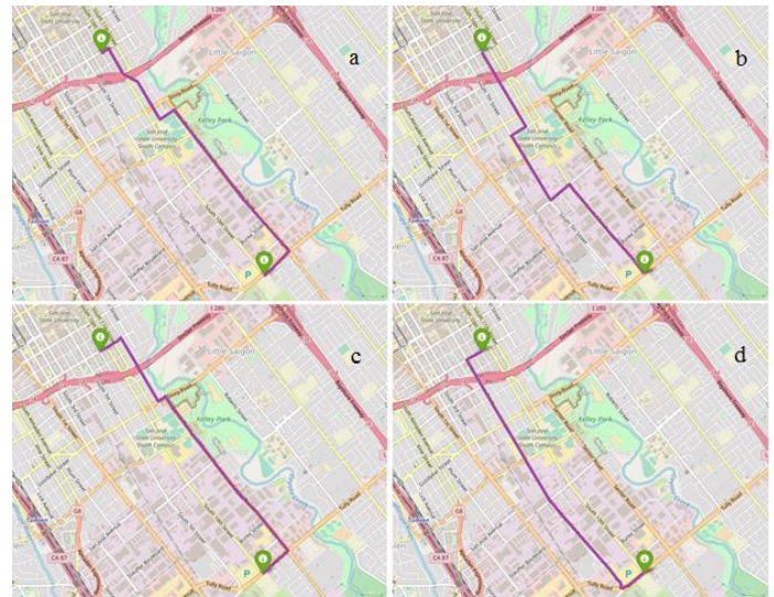
Fig 11. Optimal paths for different periods of the day (a) Optimal path during the first rush hour: 7h:00-9h:00 (b) Optimal path during the next period: 9h:00-17h:00 (c) Optimal path during the second rush hour: 17h:00-19h:00 (d) Optimal path during the next period: 19h:00-7h:00
