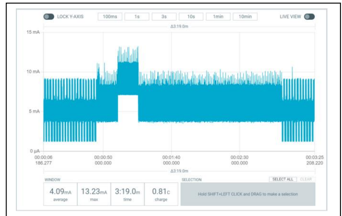
Fig. 3. Measurement of prototype device power consumption at baseline
