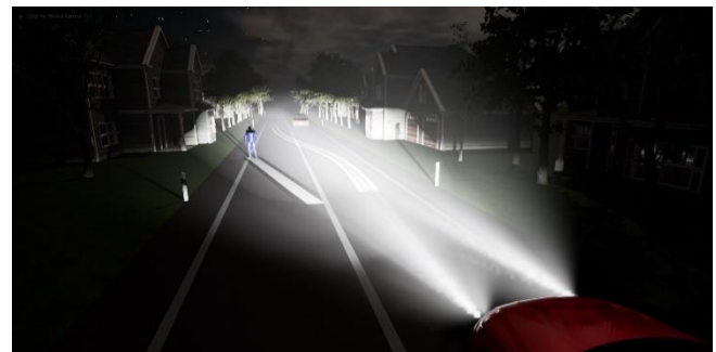
Fig. 1: Simulation of HD lighting functions such as GFHB, projecting the planned path of the automated vehicle onto the road and marking dangerous traffic objects with projected lines to direct the human driver's attention [6].
