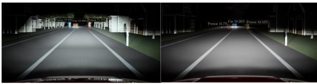
(a) High beam at 100 % usage, which would dazzle other traffic participants. (b) High beam at 8 % usage and deactivated illuminations at both sides.
