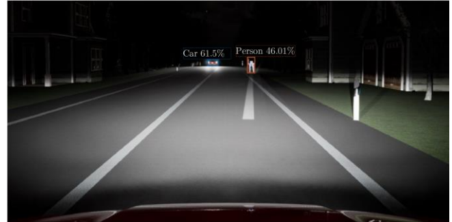
Fig. 5: Visualization of a selectively illuminated red vehicle at position p_{100,3.5} with GFHB and blue person at location p_{50,-2.5} with GFHB and marker light. The class, confidence and bounding boxes of the YOLOv5 [9] object detection are also shown.
