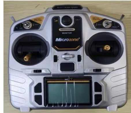
Fig. 9. The Remote control that can be used to control the motion of the robot if the control system is properly installed.
